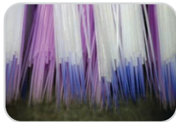
Extremely Tapered Bristles (ETB) 30x magnification
